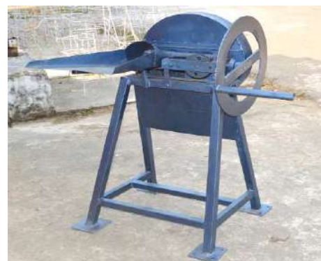
Fig: Hand operated Chaff Cutter
