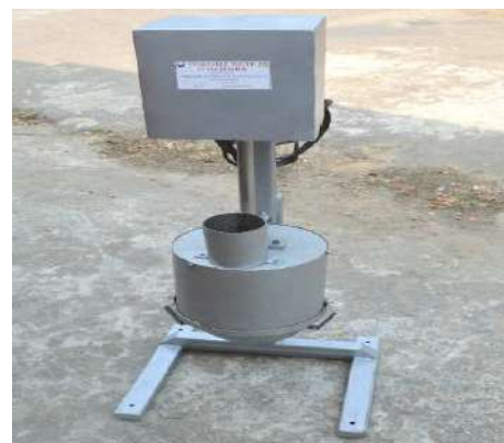
Fig: Vegetable Slicer cum crusher
